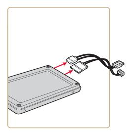
**8** Install the new hard drive and close the CV61. Use the next illustration for the tightening sequence for the back cover. Tighten the screws to a final value of 0.73 Nm (6.5 lbf-in).
