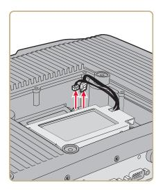
5 Remove the four screws that secure the hard drive bracket to the CV61.
