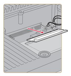
**6** Insert the new memory and close the CV61. Use the next illustration for the tightening sequence for the back cover. Tighten the screws to a final value of 0.73 Nm (6.5 lbf-in).
