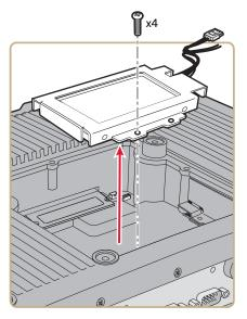
**6** Remove the four screws that secure the hard drive to the hard drive bracket.
