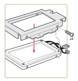
**7** Remove the two cables that are connected to the hard drive.
